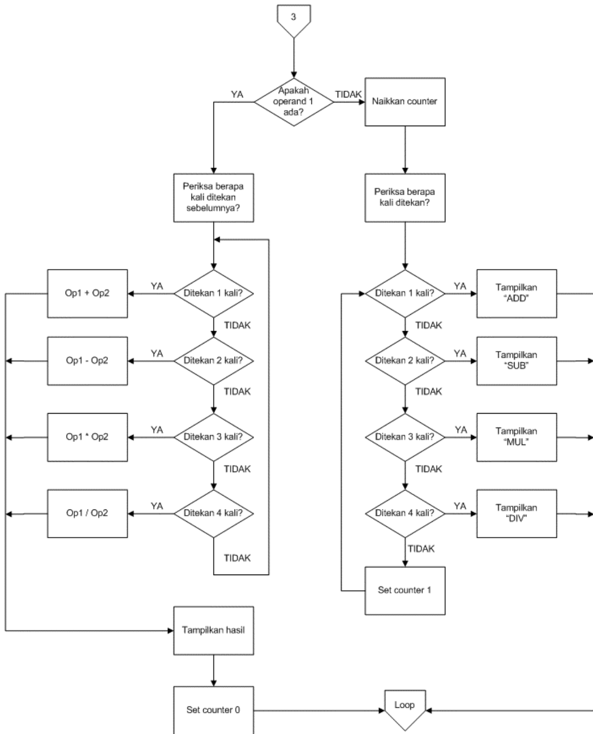
Gambar 8. Flowchart penekanan tombol spesial (proses +, -, x, /, atau =)
