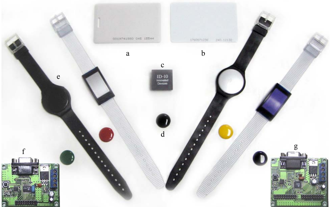
Gambar 1 ID Clamshell Card (a), Card (b), ID-10 (c), Tag (d), Wristband (e), DT-BASIC Micro System (f), DT-BASIC Mini System (g)
